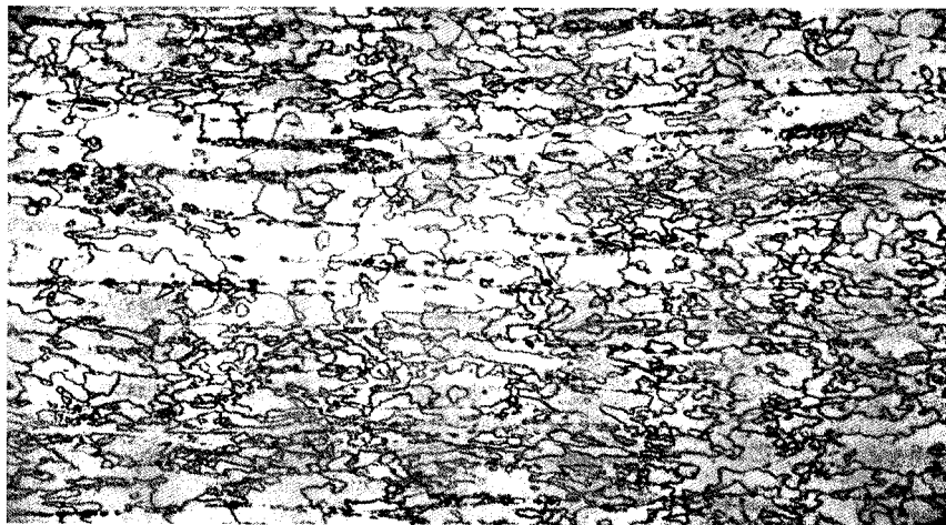
Figure 1- Grain Structure of Rolled Lead Calcium Silver Anode
